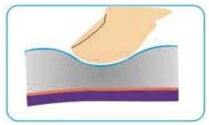
Area arrays can resolve contact position with millimeter precision and can resolve multiple contacts simultaneously. Devices can respond on a sub-millisecond timescale. Operating temperatures can range from -80°C to over 200°C depending on the choice of materials.
