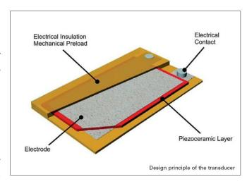
Applied directly to a substrate, or used as part of the structure itself, DuraAct<sup>™</sup> patch transducers can detect and produce vibrations or contour deformations at the source, inside the structure. The magnitude of usable deflection depends strongly on the substrate properties, and extends into the millimeter range.
